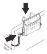
Remove the cover of the air pipe connector and connect the air pipe connector to the power unit and then ensure that the air tubes are free from any kind of obstruction, and are not kinked.
