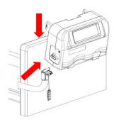
Unplug the cover of the air pipe connector and connect the air pipe connector to the power unit and then ensure that the air tubes are free from any kind of obstruction, and are not kinked.
