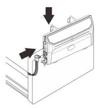
Remove the cover of the air pipe connector and connect the air pipe connector to the power unit and then ensure that the air tubes are free from any kind of obstruction, and are not kinked.
