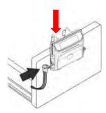
Remove the cover of the air pipe connector and connect the air pipe connector to the power unit and then ensure that the air tubes are free from any kind of obstruction, and are not kinked.
