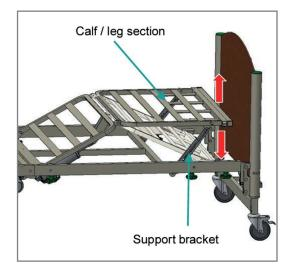
To lower the calf/leg section (from raised height), fully raise calf/leg section manually and then gently lower it down. Then press and hold the down knee-break adjustment button on the handset.
