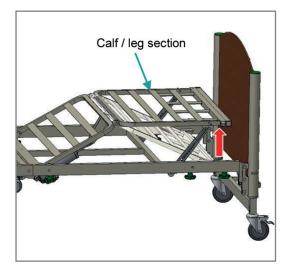
To decrease the knee break angle, manually raise the calf/leg section to the desired position. The calf/leg section will automatically lock into place.
