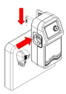
Remove the cover of the air pipe connector and connect the air pipe connector to the power unit and then ensure that the air tubes are free from any kind of obstruction, and are not kinked.
