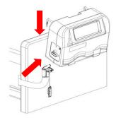
Unplug the cover of the air pipe connector and connect the air pipe connector to the power unit and then ensure that the air tubes are free from any kind of obstruction, and are not kinked.
